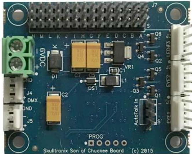
The **"Son of Chuckee"** is a DMX controlled 14 channel RC servo controller. It is THE best servo controller for use with digital and analog servos alike. And the SOC is the best controller for use with Animatronic characters. The SOC is available as a board only or as a full kit.
